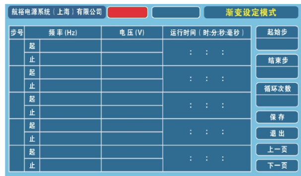
The gradient settings page can set the desired voltage and frequency. Run time, initial step, end step
