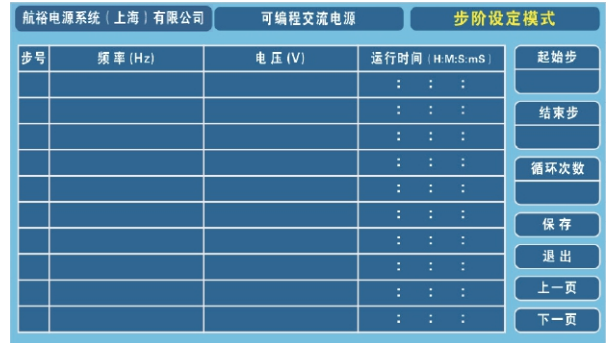
The step setting page can set the desired frequency, voltage, Run time, initial step, end step, and number of cycles
